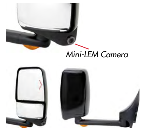
2020 Mini-LEM with turn signal option in flat glass
